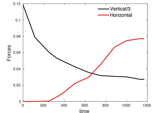
Net force is computed from Maxwell stress over outside of resistive wall.
