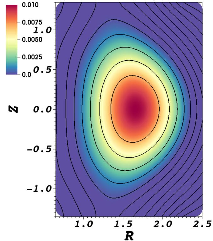
Contours of poloidal flux and pressure for the initial state. Border is the resistive wall.
