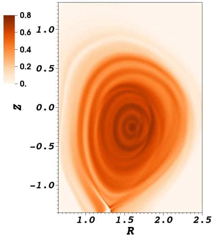
Plot of  $\langle \mu_0 J_{||} / B \rangle$  at  $t = 1373 \tau_A$  of the new simulation, where  $\langle \rangle$  indicates toroidal average.
