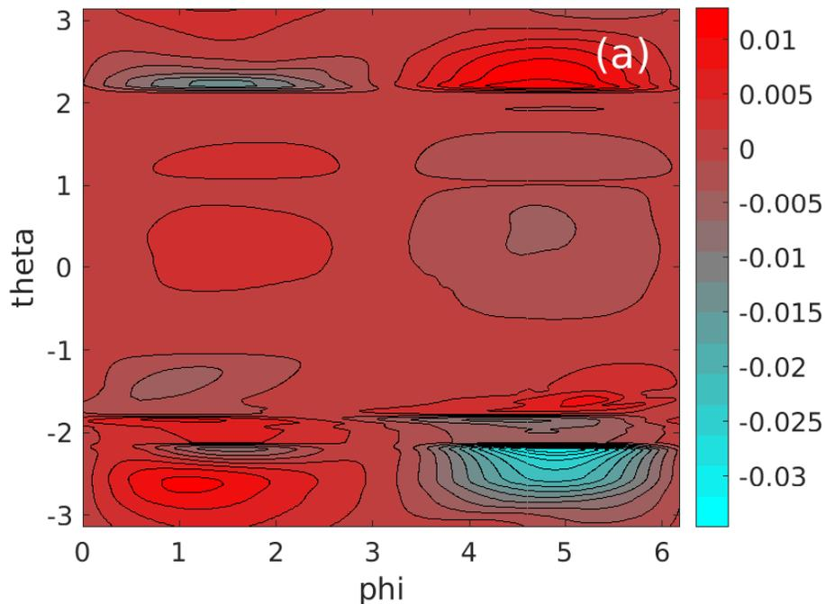
Cartesian  $y$ -component of force per unit area at  $t=971$  of the forced 3D computation.
