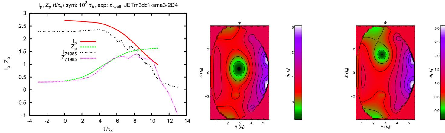
Time history plot of toroidal current  $I_p$ , and vertical displacement  $Z_p$  as function of  $t/\tau_x$ . Simulation time units  $\tau_x = 10^3 \tau_A$ , experimental time units  $\tau_x = \tau_{wall}$ .  $\psi$  at  $t = 0$  and  $t \approx 8\tau_x$ .
