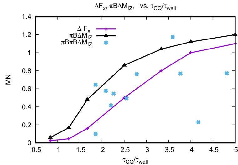
Solid curves: M3D simulations of shot 71985 where  $\tau_{CQ}/\tau_{wall}$  was artificially varied. Plots of asymmetric wall force  $\Delta F_x$  and Noll formula  $\Delta F_x \approx \pi B \Delta M_{IZ}$ .
