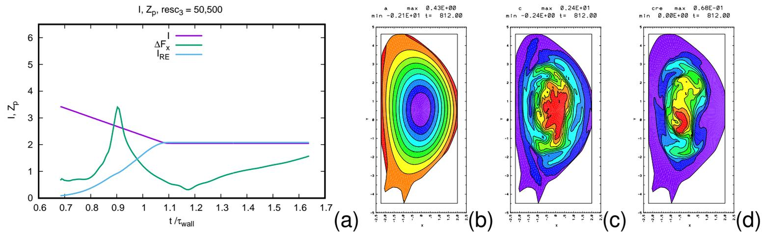
(a) Time history of RE simulation with total current  $I$ , runaway current  $I_{RE}$ , and wall force  $\Delta F_x$ . (b)  $\psi$  at  $t = 0.8\tau_{wall}$ . (c)  $J_\phi$  (d)  $J_{RE}$  at same time.
