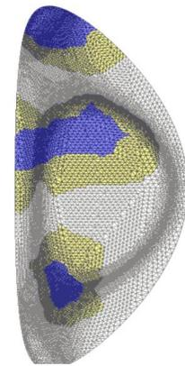
**Figure 9: Three of sixteen partitions of a mesh with ten layers of ghosted entities on each partition.**
