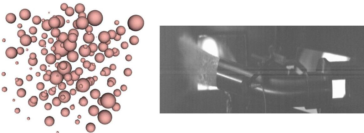
**Fig. 7: (Left): FronTier-MHD initialization of pellet debris plume for simulation of disruption mitigation in tokamaks; (Right): 16 mm neon pellet entering the shatter tube from the right at 400 m/s with the resulting spray shown exiting about 1 ms after the pellet entered the tube [100].**
